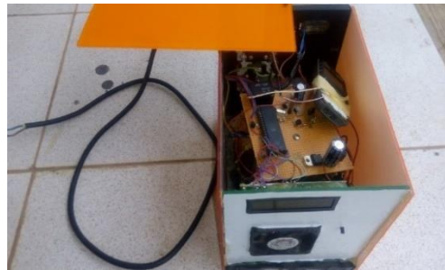
Figure 7. A Prototype of Transformer Fault Detection and Protection System
