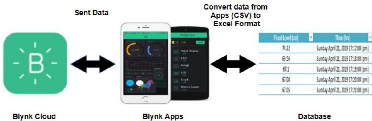
Figure 3. The Flow Database Via Blynk Apps
