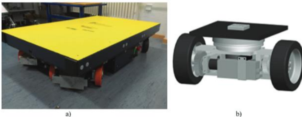
Figure 3. Multi-wheeled Mobile Platform: Mechanical Platform (a); Single Driving Module (b) [14]
