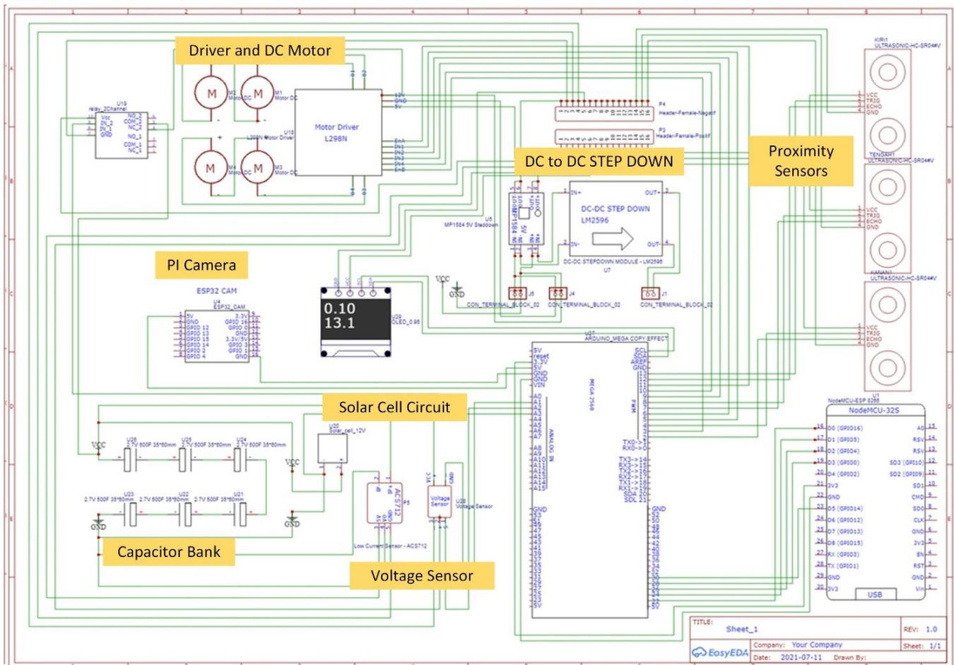
Figure 2. One-line diagrams of the surveillance robots in Figure 1
