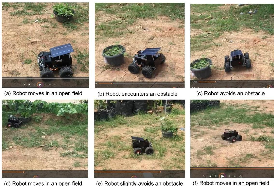
Figure 4. Surveillance robot deployment in an open field
