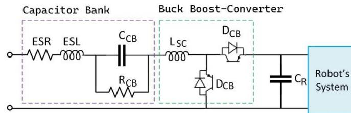
Figure 3. Charging system for the solar-power robot
