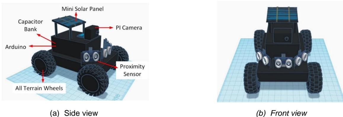
Figure 1. 3D design of the surveillance robots considered in this study
