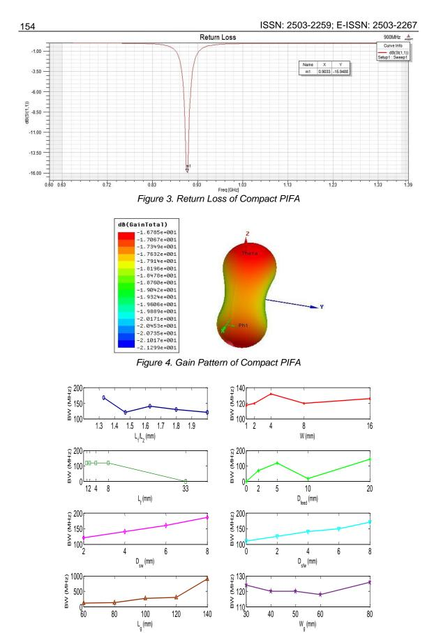
Figure 5. Plots Showing Relationship Between Bandwidth and Varied Parameters of PIFA
