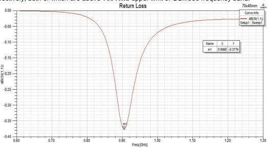
Figure 1. Return Loss of Reference PIFA
